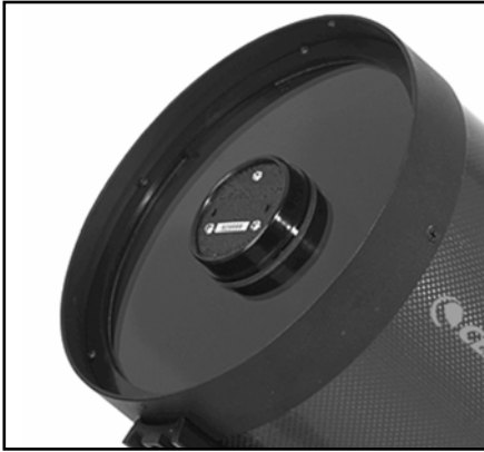
Figure 1-10 The three collimation screws are located on the front of the secondary mirror housing.
