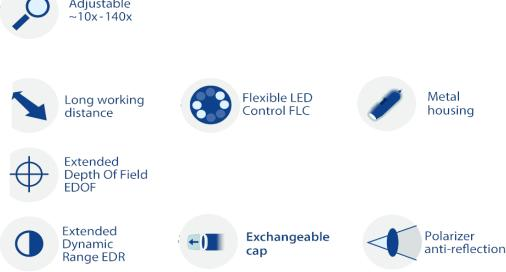
EDOF allows users to automatically capture multiple images at different depths and automatically combine them into one clear image. EDR automatically captures and combines multiple images at different exposure levels to produce a final image with greater dynamic range. The AMR function automatically detects and displays the magnification of the Dino-Lite. The magnification is displayed within the Dino-Lite software and stored with the captured picture and simplifies the measuring process.
