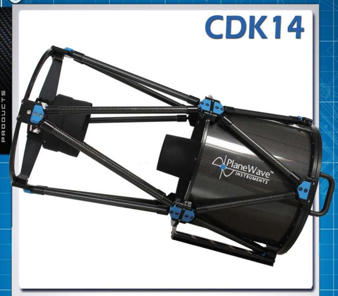
The PlaneWave Instruments CDK14 is a 14 inch (0.36 m) f/7.2 Corrected Dall-Kirkham Astrograph telescope. The CDK14 covers a 70 mm field of view without any field curvature, off-axis coma, or astigmatism. The CDK14 is a lightweight carbon-fiber truss design weighing less than 50lbs, with 3 cooling fans ejecting air from the back of the telescope. The CDK optical design is the innovative solution for unsurpassed astro-imaging quality at an affordable price.
