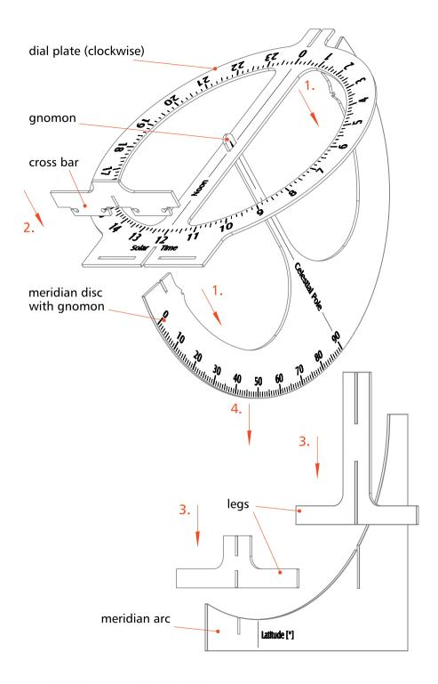
Fig. 1: Construction in four steps (northern hemisphere)
