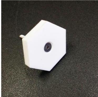
Now insert the screws with the Teflon Foot Bearings into the foot holes that you drilled out earlier. Note that you are going to **BOLT** the Teflon Foot Bearings onto the ground board. The screw (h) should slip through the ground board without you having to screw it in. **(This is why you drilled out the hole earlier using your 5/32" drill bit).**
