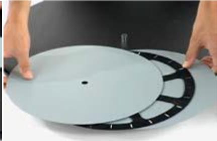
3. Leave the threaded center insert in place (it came already firmly fixed in the center hole of the ground board when purchased). Remove the two plates and the “wagon wheel” (with needle bearings) from the ground board. Set aside (they won’t be needed). Also set aside the Axle Sleeve (the plain tube resting on top of the center insert). The Axle Sleeve won’t be needed.
