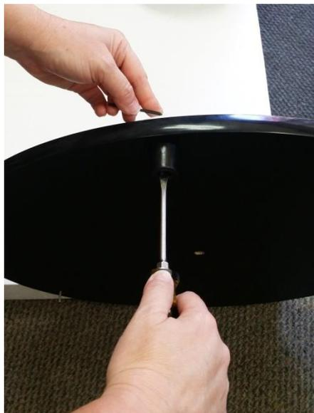
7. Now gently tighten the assembly until it is just snug by turning the screw (h) with the included 3/32 Hex Wrench (k) while holding the 8-32 Nylon Insert Lock Nut (j) still. You will find that there is no easy way to get a socket in there or otherwise hold the lock nut while turning the screw. But this is a good thing because it will prevent you from overtightening the screw and
