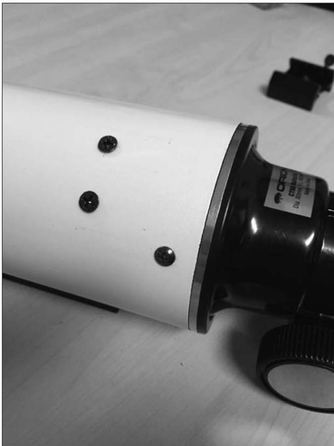
Figure 6. Reinstall the screws, nuts, and focuser
