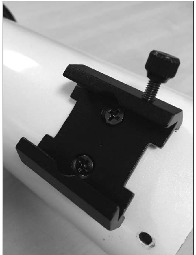
Figure 4. Finder bracket screws
