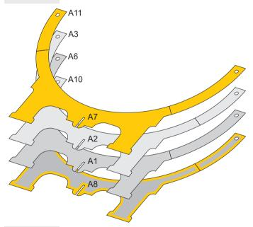
**Step 1:** Glue the two inner parts of the north/south support [A1, sheet 15 + A2, sheet 16] flush on top of each other, with the front sides facing each other. The parts are asymmetrical, so there is a tag protruding on each side.
