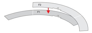
**Step 24:** Glue the meridian inner parts 1 and 2 [F1, sheet 5 + F2, sheet 6] together on their designated glue marks with their front sides facing each other, as depicted. Both parts have a cutout on their inner edge that will later receive the equinoctial. Make sure that these cutouts are exactly flush. The parts overlap on two thirds of their length, one third protrudes on each side.
