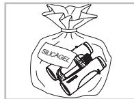
If the instrument is wet, it must be dried prior to storage.
