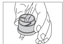
In the event of hard-to-remove dirt (e.g. sand) the eye cups can be unscrewed and cleaned very easily.
