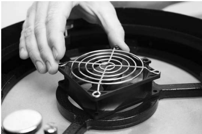
Figure 1. Line-up the holes in the fan and fan cover with the holes in the rear of the mirror cell.
