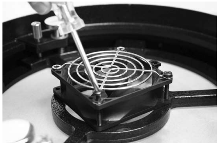
Figure 2. Attaching the fan to the mirror cell.
