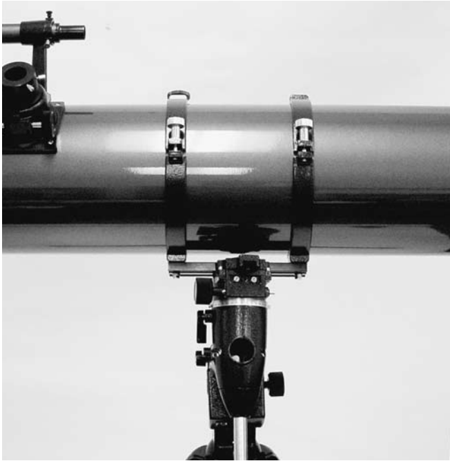
Figure 11. The optical tube must be at a 90° angle to the right ascension axis in order to view through the polar axis finder
