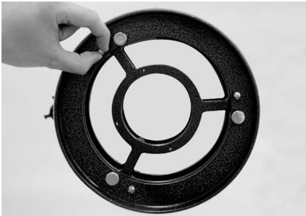
Figure 17. The three small thumbscrews that lock the primary mirror in place must first be loosened before any adjustments can be made.
