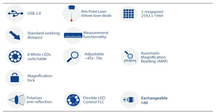
The AM7515MTFP is part of the Long Working Distance (LWD) range and with its Long Working Distance and magnification range from 45-70x, it is suitable for a wide range of applications where extra distance to the object or a larger field of view is required.
