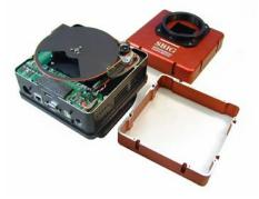
2. Remove the front cover of the filter wheel and the front cover of the camera. Re-use the 8 screws from the camera front cover to attach the red spacer that you previously removed from the back plate of the filter wheel.
