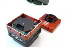
3. Attach the filter wheel base to the red spacer that is attached to the camera body. At this point you should install the filters if not already installed.
