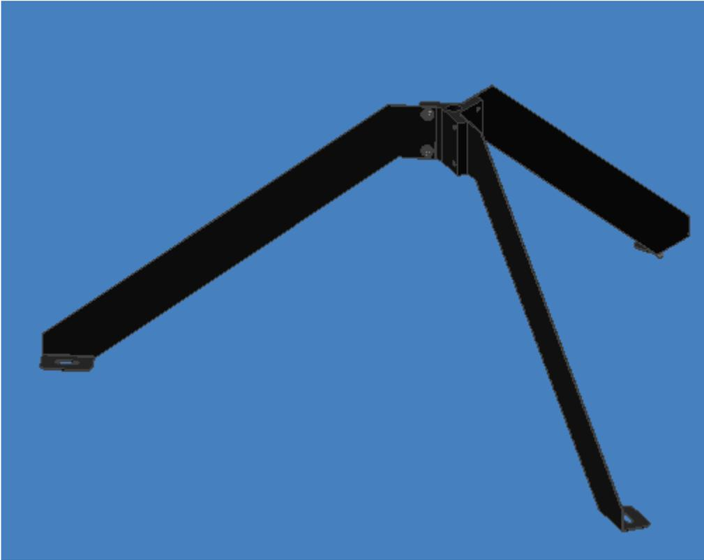
**Figure 8: Attach the three spider wings to the spider hub**
