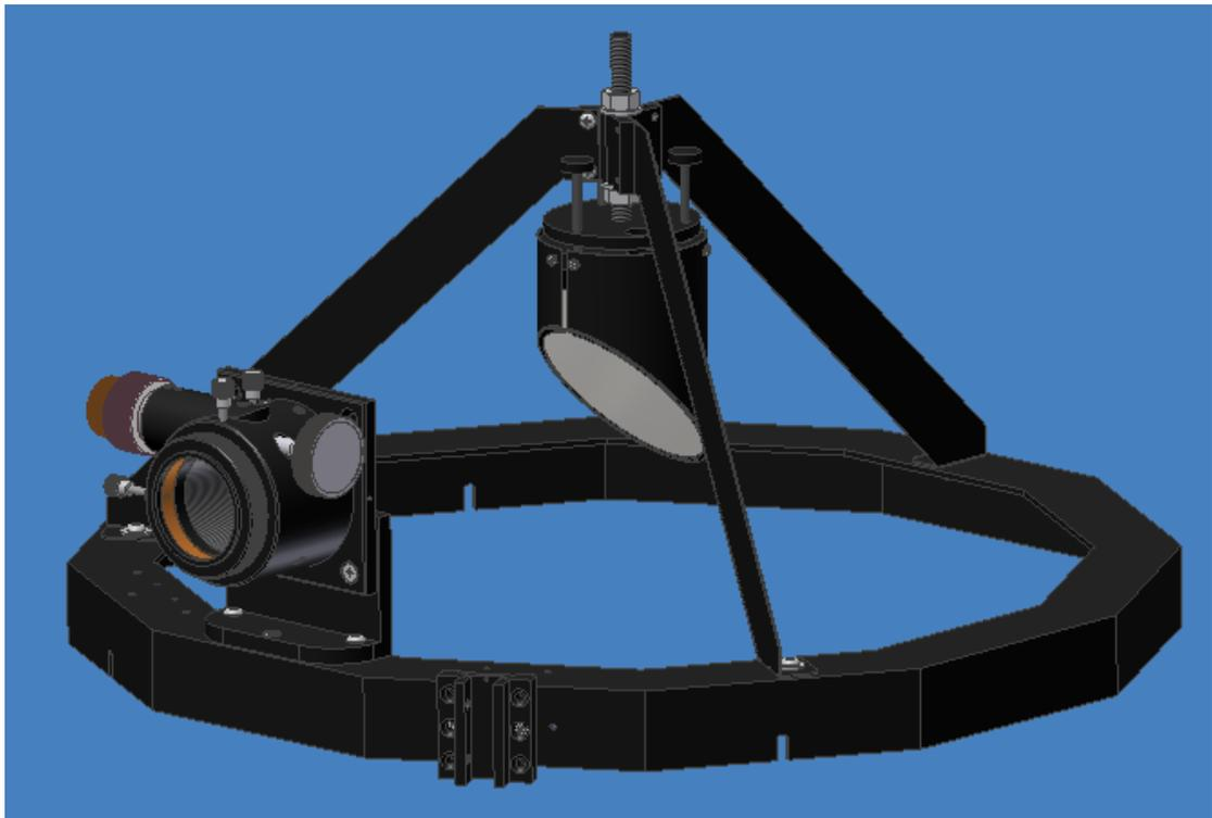
**Figure 12: Attach the secondary holder with the secondary mirror**
