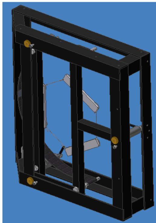
Place the two spacers around the ALT bearing installation holes. (Please note that the spacers are already installed).
