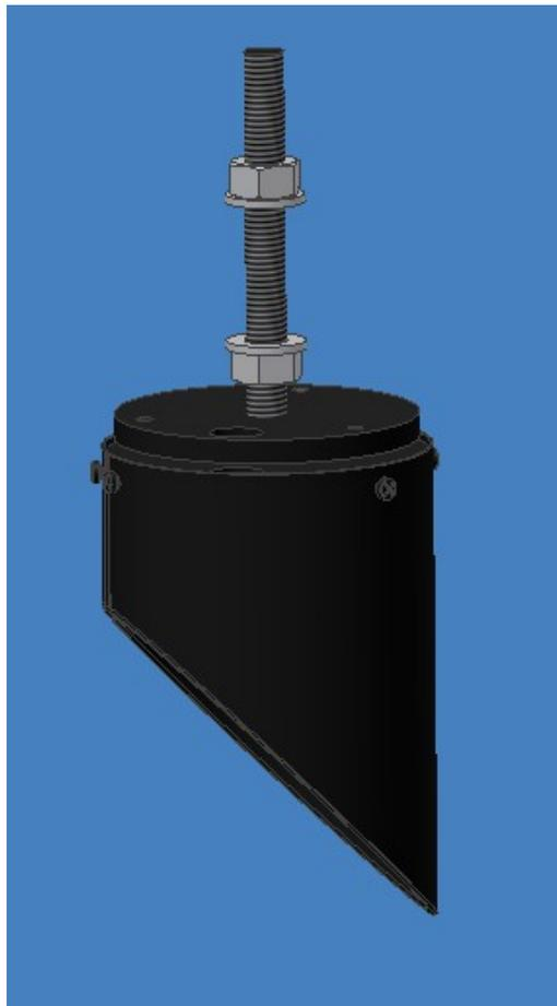
**Figure 4: Secondary Spider Hub/ Diagonal Support**
