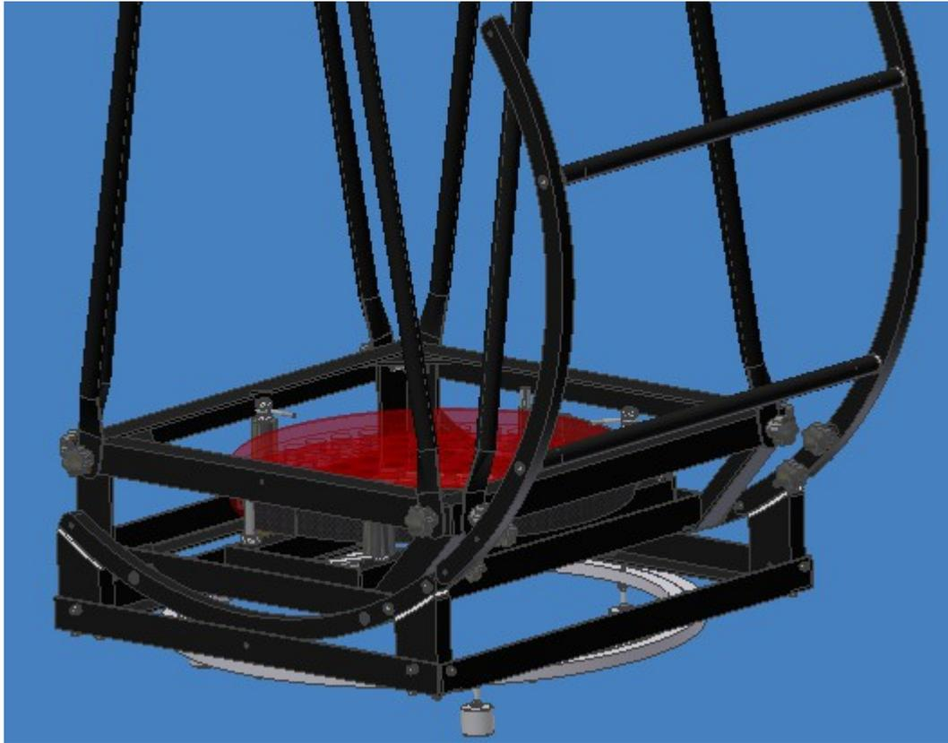
**Figure 18:**Tighten the knob screws
