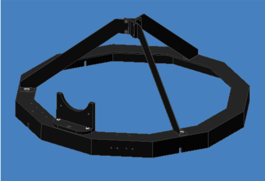
**Figure 10: Attach the focuser L bracket to the upper ring**
